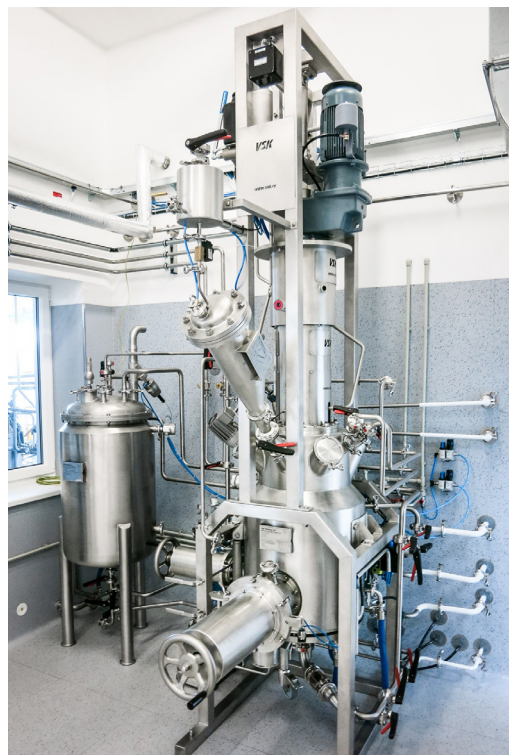
Filter dryer of 100 liters volume, pharma version ATEX
