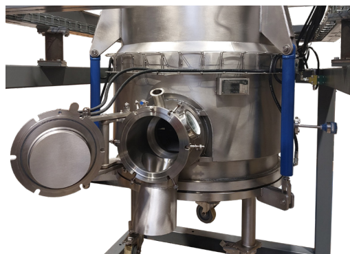
Detail of the open discharge valve
